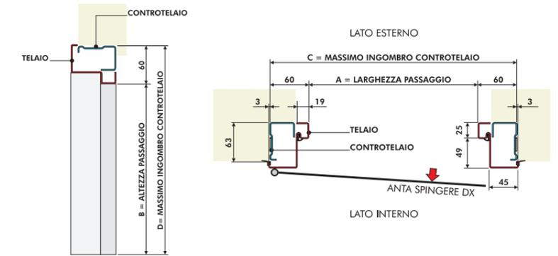
MISURE STANDARD PER IL TELAIO E CONTROTELAIO
